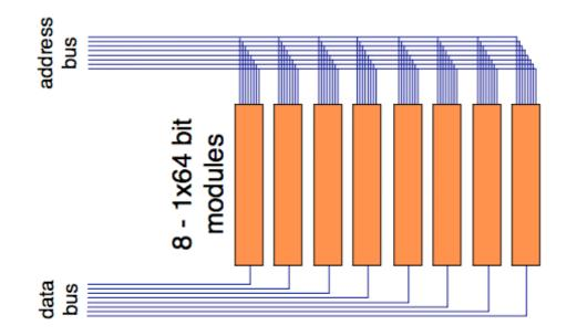
Figure RAM2. The eight one-bit RAM chips that make up this module share row and column address lines. The top 4 lines of the address bus specify the row while the bottom 4 lines specify the column . The row and column data from the bus is decoded on each chip to select the bit at row 2 and column 6 (see Figure RAM1). The data sent on the data bus is not decoded, it just sets the status of the corresponding bits on each chip.
